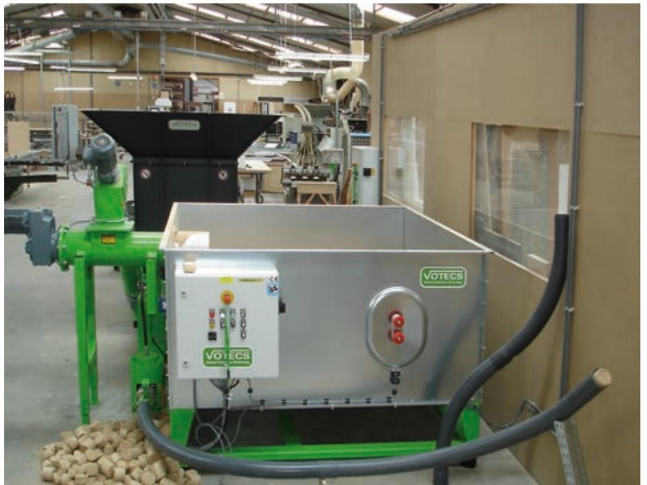
Depending on the material, the briquetting press „AP 775“ enables hourly capacities of 120 to 160 kg.
