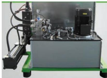
The hydraulic tank is arranged separately. In this way, the emerging oil heat is optimally discharged. Easy access makes the regular maintenance service pleasant and efficient.
