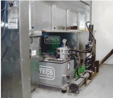
Left: Briquetting Press AP 555 installed under filter system.
